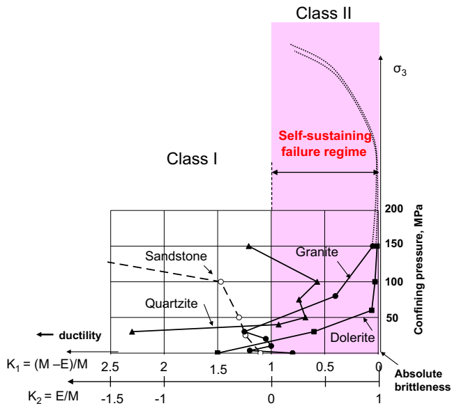
Fig. 11. Variation of brittleness indices K_1 and K_2 versus confining pressure \sigma_3 for rocks of different hardnesses (modified from [1–3]). (For interpretation of the references to colour in this figure caption, the reader is referred to the web version of this article.)
